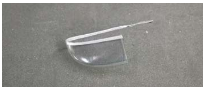
More aluminium strips being formed around the wing tips clear plastic cover
