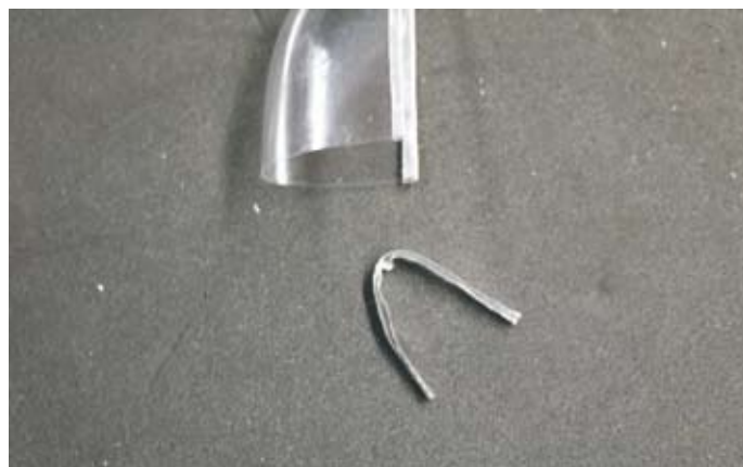
Aluminium strip being pressed around the wings tip clear cover using the wing tip clear cover as the template
