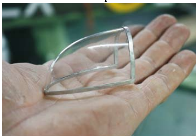
Aluminium strips are glued in place to the wing tips clear plastic cover using canopy glue
