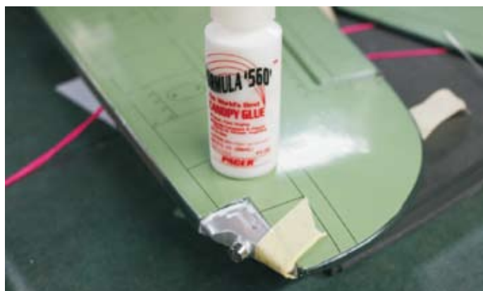
LED and wing tip vacuum formed housing being glued down with canopy glue.
