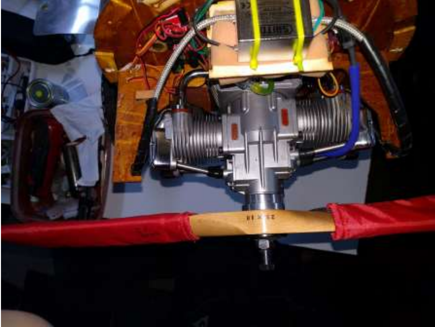
Insert Photo 9 Top view of the baffles, note the gap on the outside of the baffle with respect to the fuselage diameter, this is filled in with the foam that is mounted in the cowl. This was designed this way so that the cowl could be easily removed and that this space was filled in to stop the passage of air.
