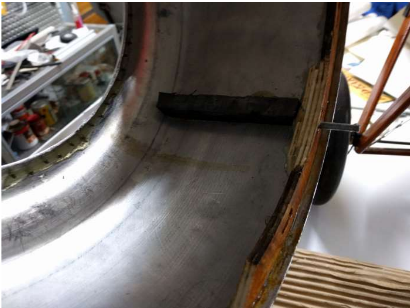
Insert Photo 2 Cowl mounting bolt fixed to ply ring. Note: foam mounted in the cowl to prevent the air taking the easiest path out past the internal baffles
