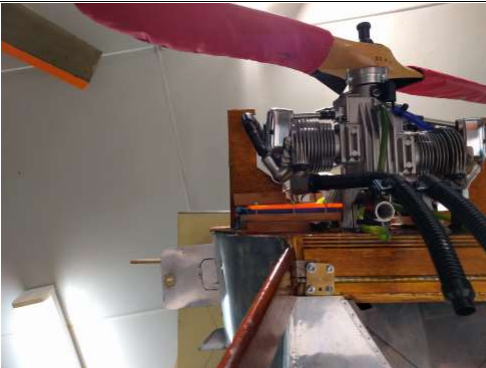
Insert Photo 8 Bottom view of the baffles around the engine cylinders.
