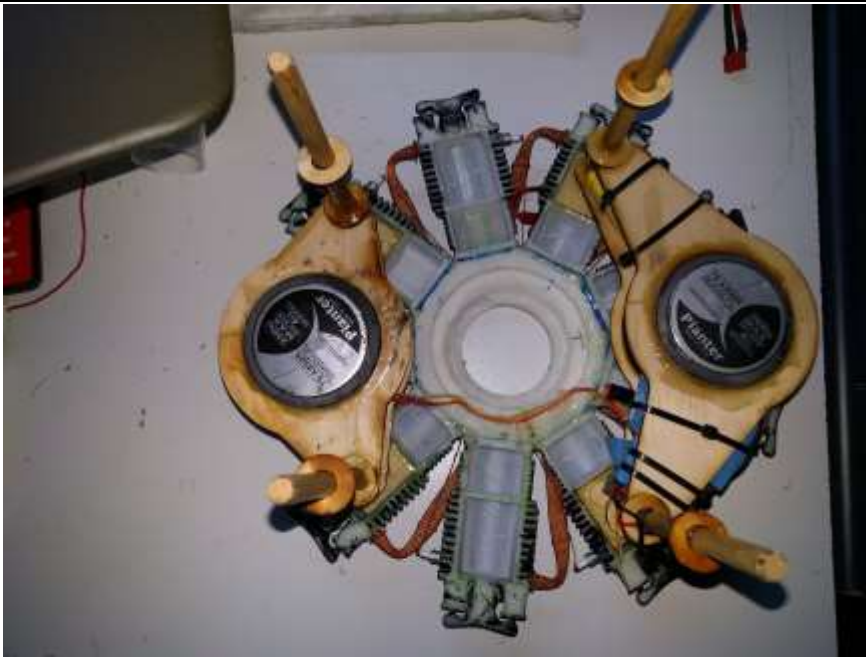
Insert Photo 7 2 x 200 watt speakers mounted to the dummy engine along with audio board and amplifier.
