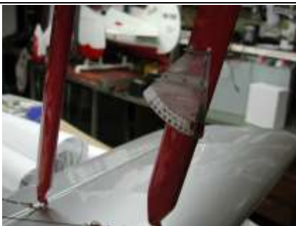
Picture: Air speed indicator fitted to left hand side front strut.
