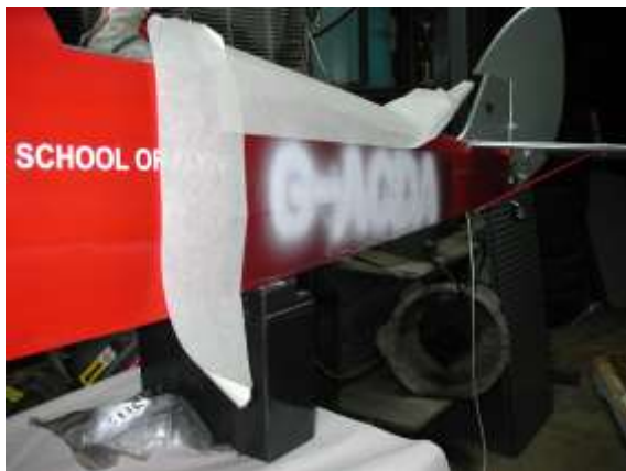
Picture: Recovering using Acetate and painting the fuselage
