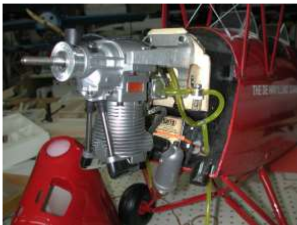
Picture: Magnificent Saito FG-36cc Petrol motor mounted inverted in the Tiger.
