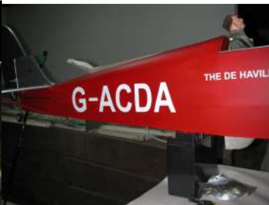
Picture: Recovering using Acetate and painting the fuselage
