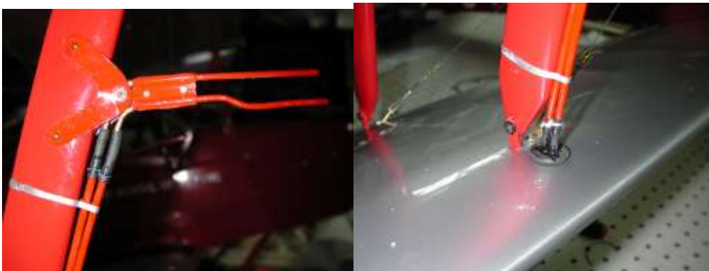
Picture: Pitot air speed indicator fabricated using aluminium sheet and copper tubing.
