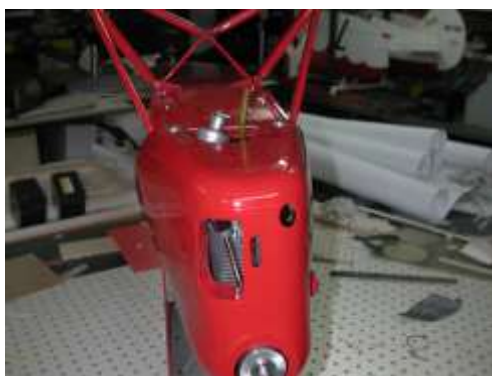
Picture: Nice view of the Saito engine, almost looks like the de Havilland Gypsy Major from the front with the pushrod tube visible.
