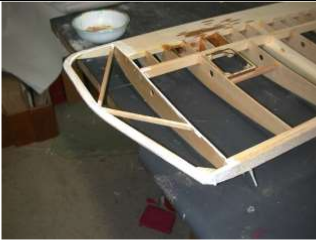
Insert Photo 10 Glue applied to wing tip
