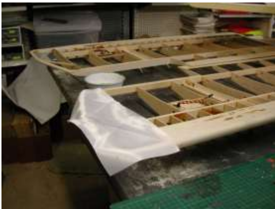
Insert Photo 11 Covering wrapped over glue
