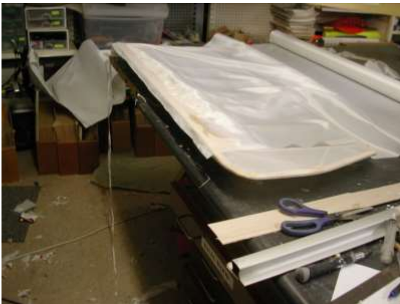
Insert Photo 15 . Cloth glued to leading edge and ready to do the total wrap around.
