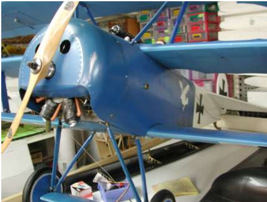
Picture: 1/4 scale DR1 dummy engine and machine guns made from cardboard.
