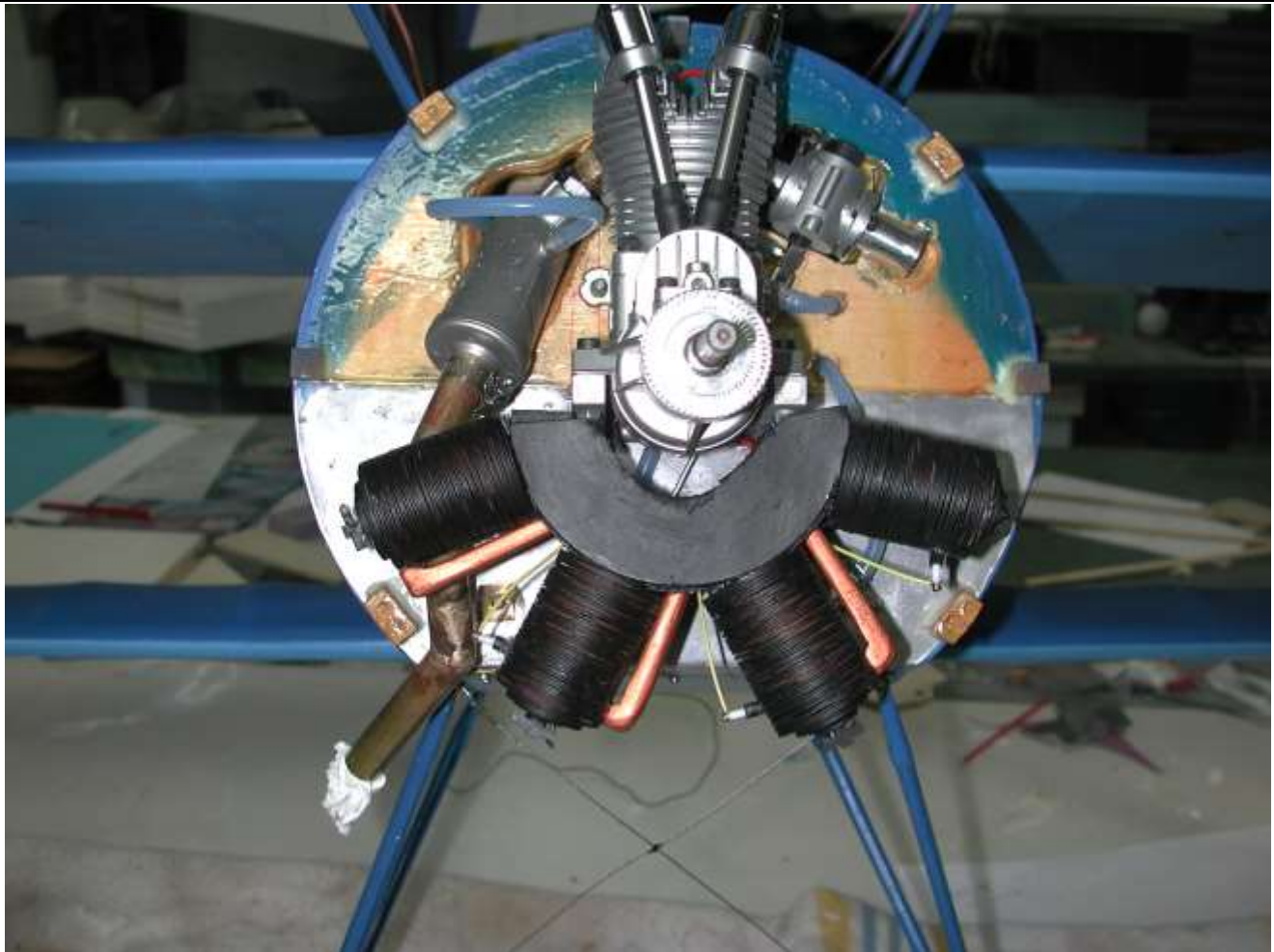
Picture: Dummy engine fitted on dowel rods. ¼ scale DR1 powered by Saito 180.
