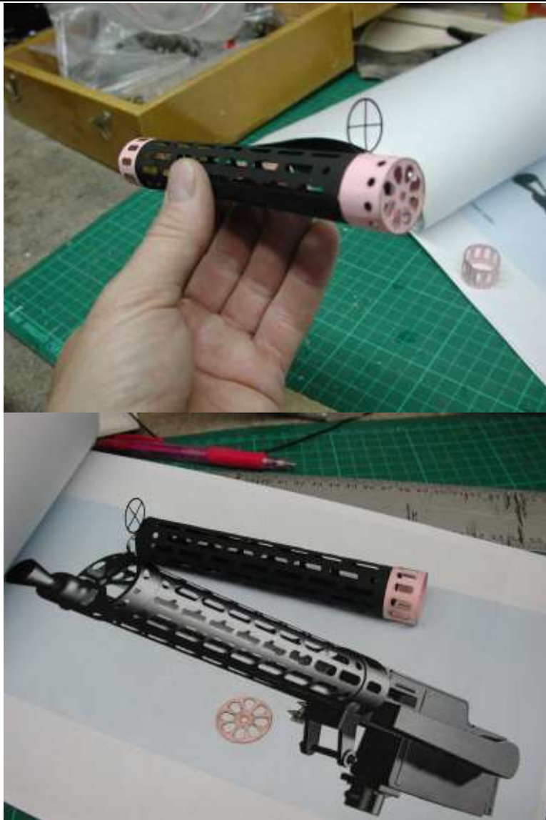
Picture: Barrel completed, light and robust. The gun sight is also made from laser cutting cardboard and then coated with thin CA and painted with acrylic paint to provide greater strength.
