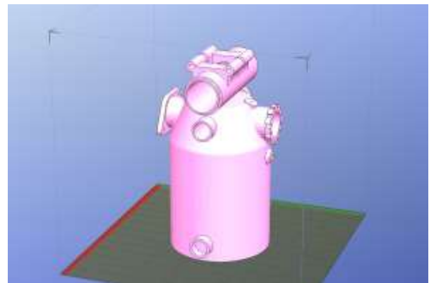
Picture: D111 cylinder draw using CAD system and then the STL file is generated and loaded into the 3D printer software to control the 3D printing process.
