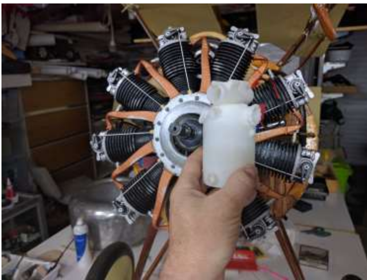
Picture: 1/3 scale Mercedes D111 cylinder compared with the Le Rhone 1/3 radial engine that I made for the Sopwith Pup.
