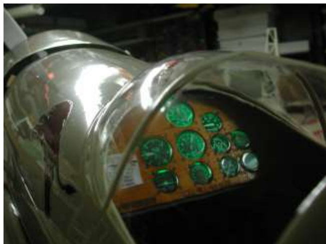
Picture: Completed custom instrument panel for the Wedell Williams racer with the gauge illumination on.
