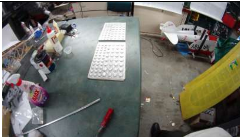
Picture: CNC machined instrument gauge forms made from aluminium. One set has rounded gauge faces of various sizes and the other one has a more square edge profile. These forms are used in the vacuum former to make the instrument clear faces in large quantities.
