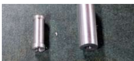
Saito engine standoff on the right is 40mm long but the ones I used are on the left at 30mm
