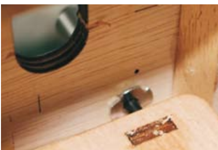
Blind nuts used on the bottom of the firewall needed to be cut to provide clearance
