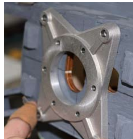
Backplate removed and used as a template for the engine mounting
