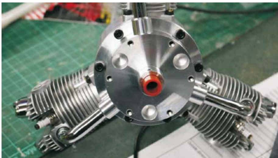
Backplate removed and used as a template for the engine mounting
