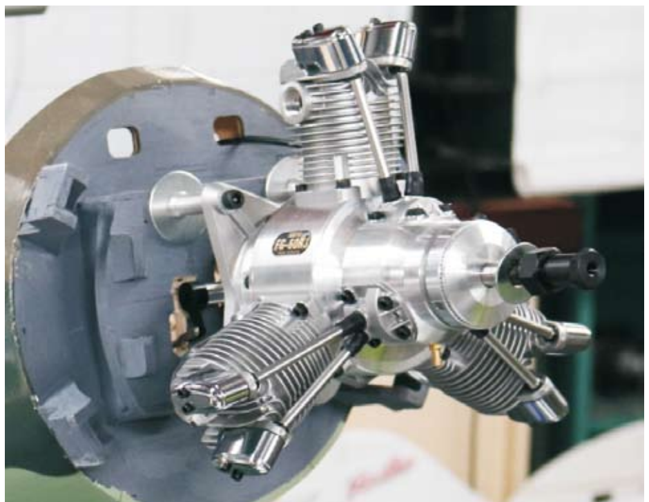
Saito triple mounted to the Lysander very neatly. Large flat washers used to reduce the crush on the firewall
