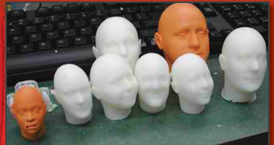
Using photo-based applications you can take photos of people's faces and generate STL files from multiple photos. Results are outstanding and heads can be printed in any scale required. You can also mess with the face parameters and generate very interesting results.
