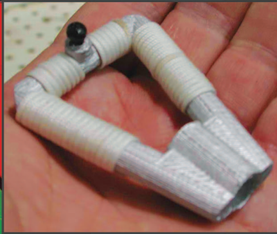
Functioning control column and handle drawn up using CAD and printed on the 3D plastic printer.
