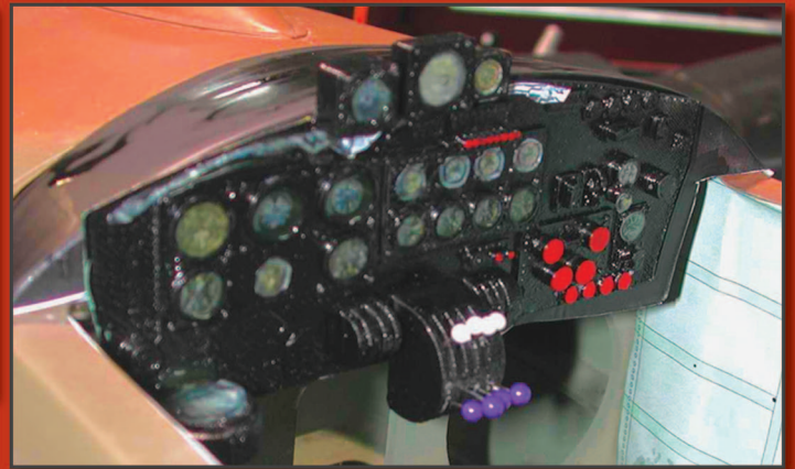
Above and Right: Something different. Lancaster instrument panel drawn up and printed on the 3D printer.
