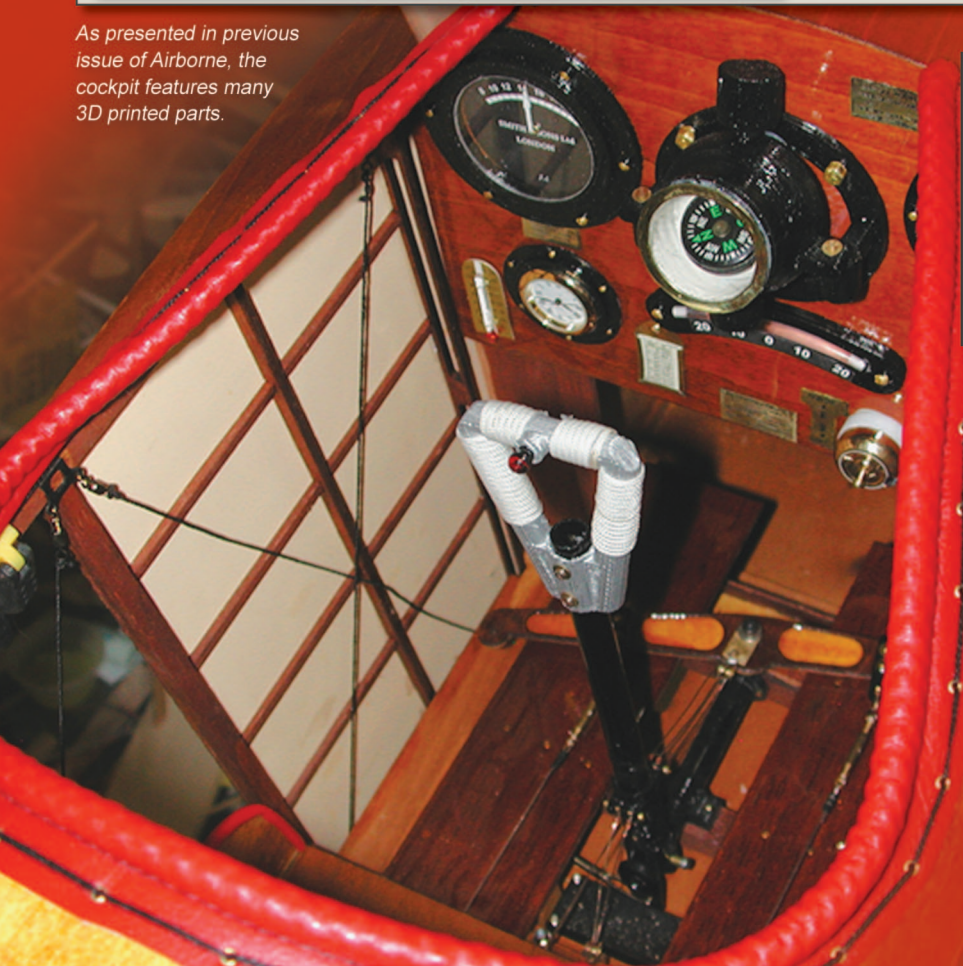
Functioning control column and handle drawn up using CAD and printed on the 3D plastic printer.
