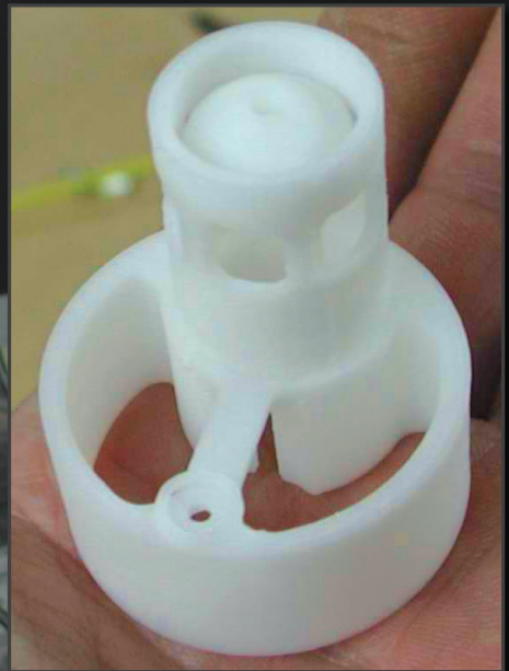
Completed ABS muzzle for the 1/3 scale Vickers machine gun.
